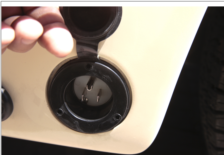
Illustration 14: Typical charging plug used on electric vehicles
