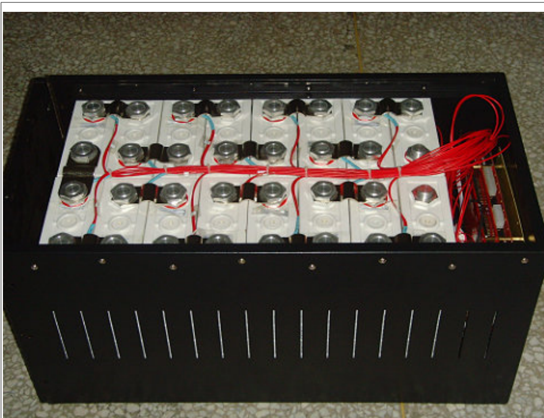
Illustration 1: Example of 16, LiFePO 4 prismatic cells with BMS
